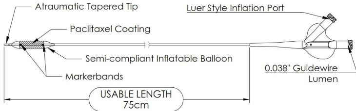
Figure 1-1. Optilume DCB Design
