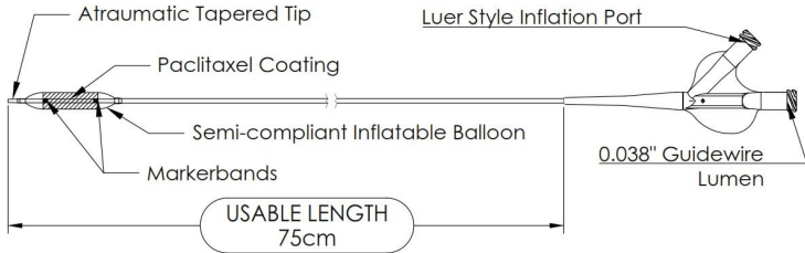
Figure 1-1. Optilume DCB Design
